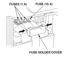
5. Install the fuse holder cover and the battery maintenance cover in the reverse order of removal (see page 56).
