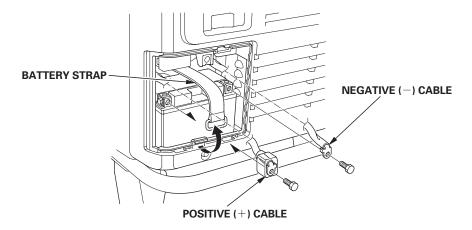
5. Remove the battery from the battery tray.
