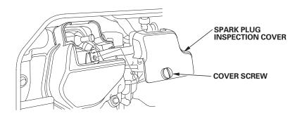
3. Disconnect the spark plug cap, and remove any dirt from around the spark plug area.
